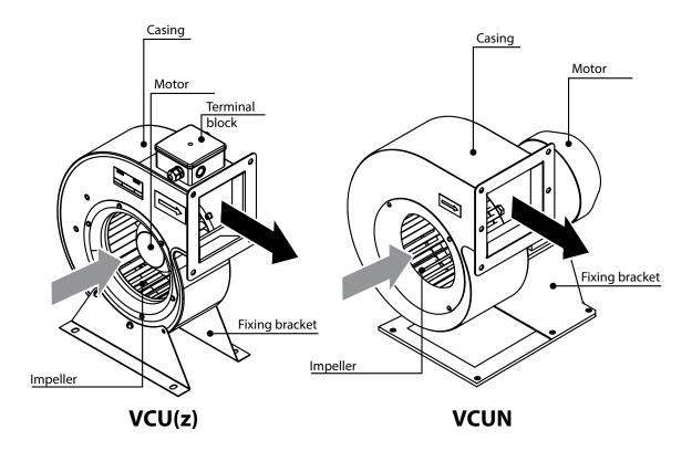
The **VCUN** fan is enclosed in a metal casing. The electric motor and the air intake ring are fixed to the casing through the flange. The impeller is fastened to the drive shaft.
