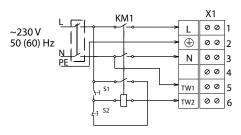
QF: automatic circuit breaker KM1: magnetic starter S1, S2: control buttons
