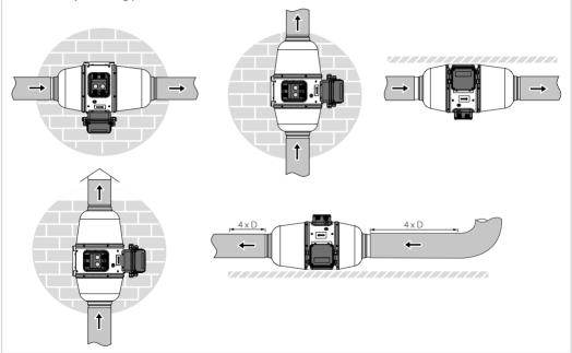
Cut off power supply and make sure electricity has been Lead the power cable to the ventilation hole, drill the turned off. Mark the holes for fixing the fan and the power mounting holes and install the dowels. cable For any mounting position: connect an air duct on both Fix the fan with the screws. sides of the fan.
