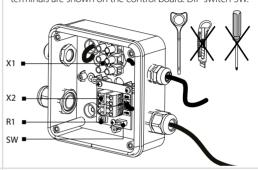
Connect the X1 and X2 terminal block counterparts. Reassemble the fan in the reverse order.
